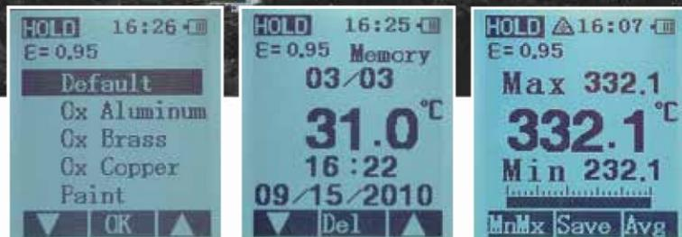
Adjustable Emissivity      Data Record      Fast measuring with high accuracy
